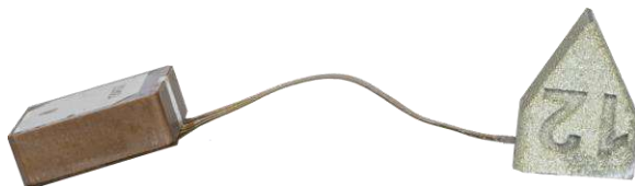
(Flexible Sensor embedded by additive manufacturing)
